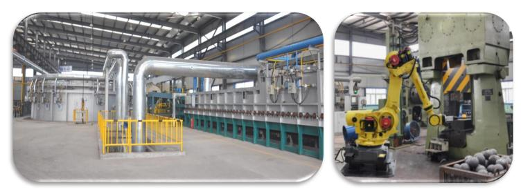
Balls are manufactured with **independent machinery** using a roll forging method with a variety of heat treatment techniques depending on the final product requirements.
